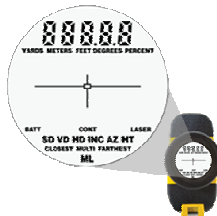
Trupulse Laser Rangefinder displaying data in scope
